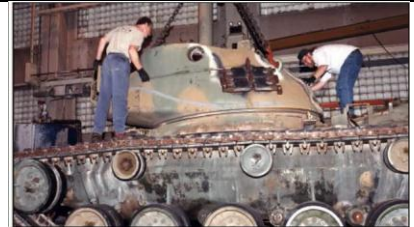
Tracked Vehicle.jpg M60A3 Tank converted to simulate Russian BMP Infantry Combat vehicle for training purposes
